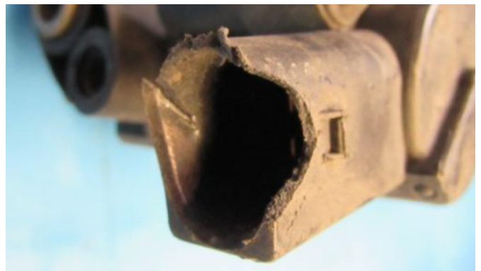
Damaged plug (valve)
