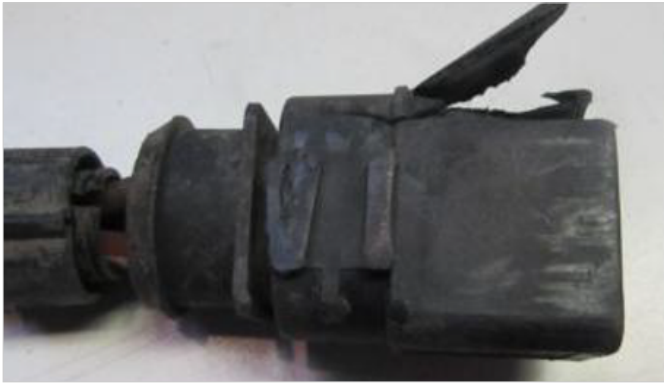
Damaged plug (wires)
